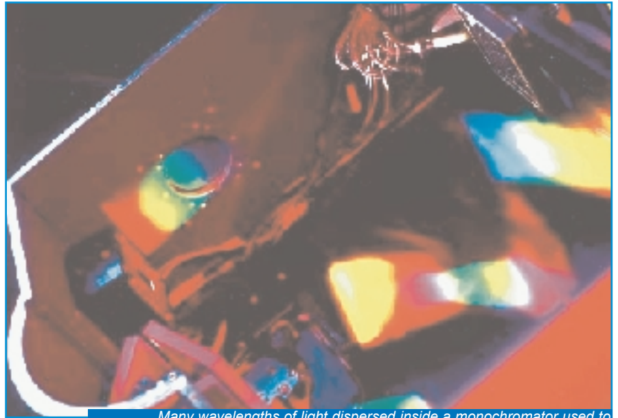
Many wavelengths of light dispersed inside a monochromator used to create two-dimensional time- and wavelength-spread codes which take full advantage of the broad low-loss bandwidth of optical fibre.
