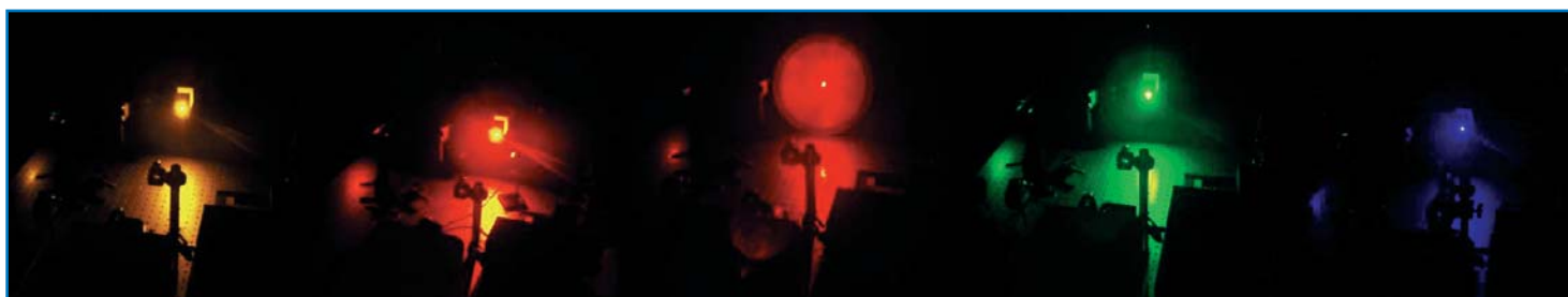
Optical parametric amplifier (TOPAS), pumped by a Ti-Sapphire regenerative and multipass chirped pulse amplifier (TITAN). (Output avg. power: 20 - 400 mW, WL range 280 nm - 2,6 um, Rep rate: 1 kHz tun., Pulse width: fs-ps).
